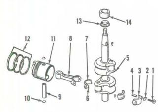
When assembling, observe the following: Piston should have long, sloping side of head (EX-Fig. OM4-12) toward exhaust side of cylinder and oil hole (H) in connecting rod should be up. Piston pin should be installed from the loose (L) side of piston. Ends of piston rings must engage pins (P) in grooves. NOTE: Only two pins are shown, pin for center ring is on other side of piston.
