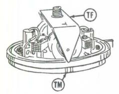
Fig. OM4-6—View of motor with timing fixture (TF) installed. Breaker points should just open when pointer is centered between timing marks (TM) on armature plate.
