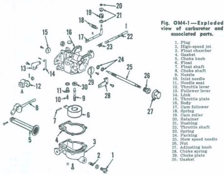
tor body (16) and check the natural position of float with body inverted. Upper surface of float (6) (lower surface with body inverted) should be level and flush with gasket surface of carburetor body. If it is not, carefully bend float lever; then check after assembly to be sure float does not bind or rub.
