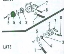
Fig. OM4-5-Fuel pump, fuel filter and associated parts. Early type pump is shown at top.
