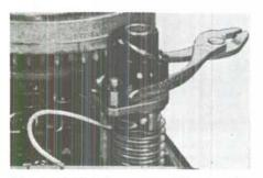
Fig. OM4-14-The starter pinion can be blocked up as shown for removing starter rope.
