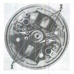
Fig. OM4-10—The magneto armature plate can be lifted off after removing the four screws (X).
