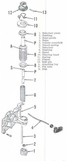
Fig. OM4-15-Exploded view of recoil starter and associated parts. Intake manifold (5) contains the mounting bracket for starter unit.
